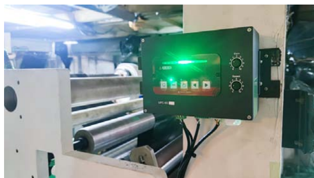
Controller Series UPC-93S is installed on Laminating Machine
